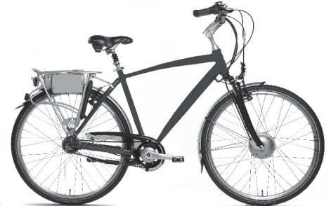
Electric motor integrated into the front hub
